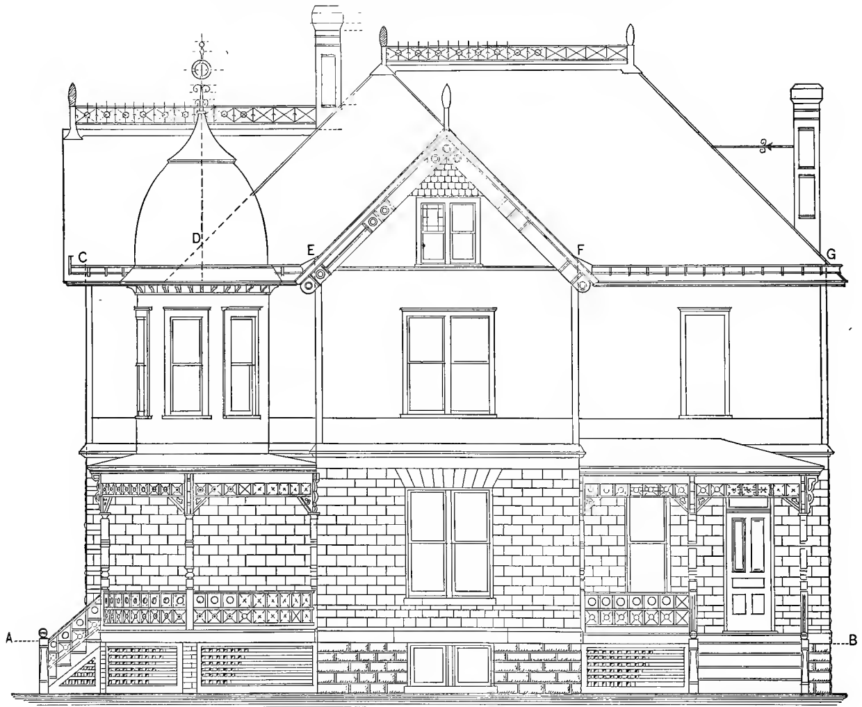
Fig. 39.—Side (Right) Elevation, Showing Parts of the Work in Different Stages of Completion.—Scale, \frac{1}{4} Inch to the Foot.
